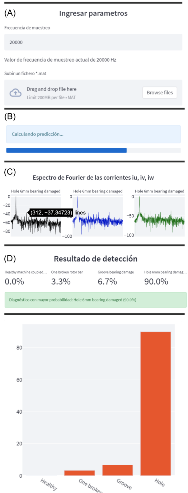
Fig. 4. GUI interface of the induction machine diagnostic system. (A) Acquisition of current signals, (B) preprocessing and prediction calculation, (C) Visual inspection of frequency spectra and (D) Global diagnosis of the current signal.
