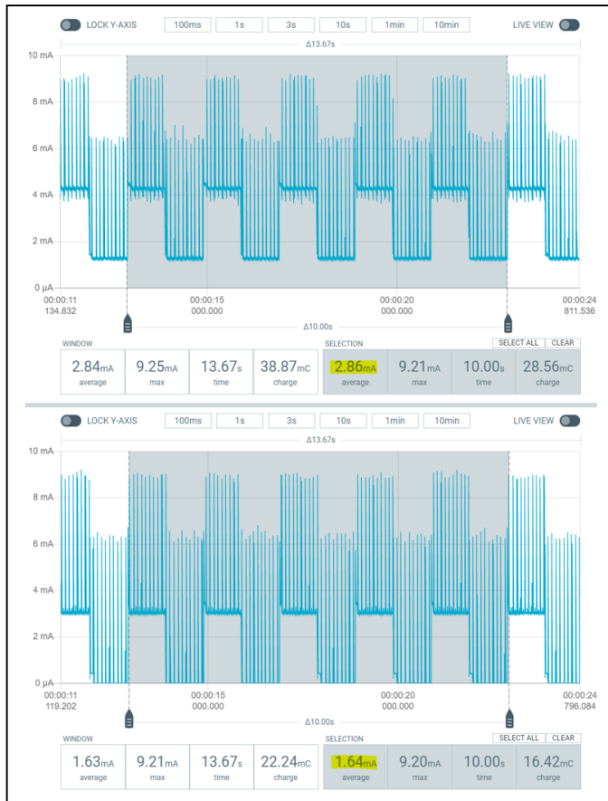
Fig. 4. Prototype device in Bluetooth advertisement mode before and after disabling serial and logging
