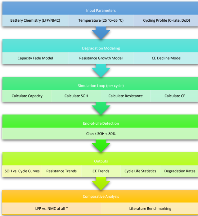
Fig. 7. Simulation Framework for Comparative SOH Analysis of LFP and NMC Batteries Across Temperatures
